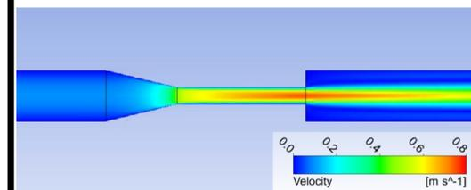
Fig. 5 – CFD velocity prediction (current study) showing flow acceleration in the throat and subsequent jet diffusion
