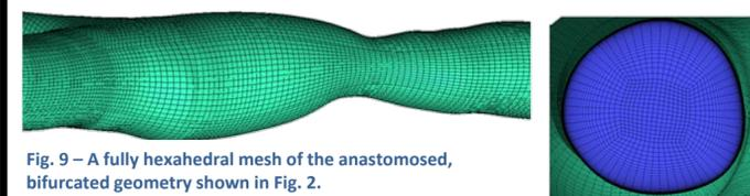
Fig. 9 – A fully hexahedral mesh of the anastomosed, bifurcated geometry shown in Fig. 2.
