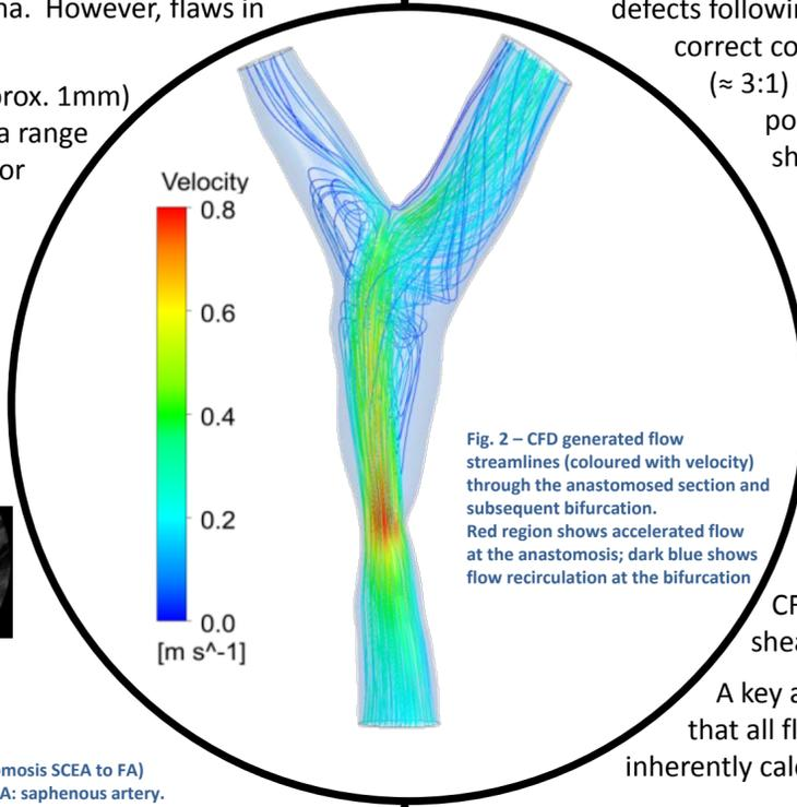
Fig. 2 – CFD generated flow streamlines (coloured with velocity) through the anastomosed section and subsequent bifurcation. Red region shows accelerated flow at the anastomosis; dark blue shows flow recirculation at the bifurcation
