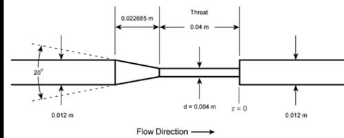
Fig. 3 – The idealised geometry of the FDA's first Computational Inter-laboratory Study (from Stewart *et al.* [3])
