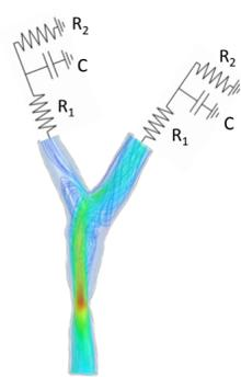
Fig. 7 – The commonly used Windkessel boundary condition applies resistances and capacitances to represent downstream vasculature
