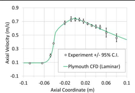
Fig. 6 – Comparison between current study and FDA experimental results: Axial velocity at the centreline for  $Re_{throat} = 500$
