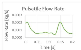
Fig. 8 – The experimentally measured transient flow rate used in [2]
