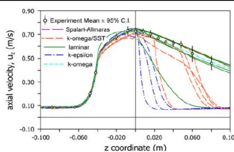
Fig. 4 – Results from the FDA's first Computational Inter-laboratory Study: Axial velocity at the centreline for  $Re_{throat} = 500$  (from Stewart *et al.* [3])
