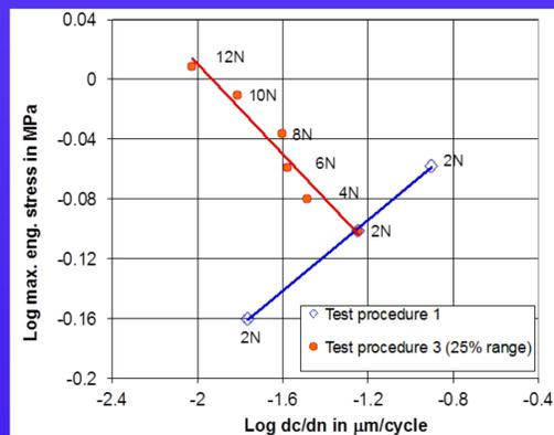
Crack propagation rate results for carbon black filled EPDM, showing maximum stress dependence.
