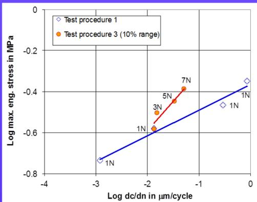
Crack propagation rate results for unfilled EPDM, showing maximum stress dependence.
