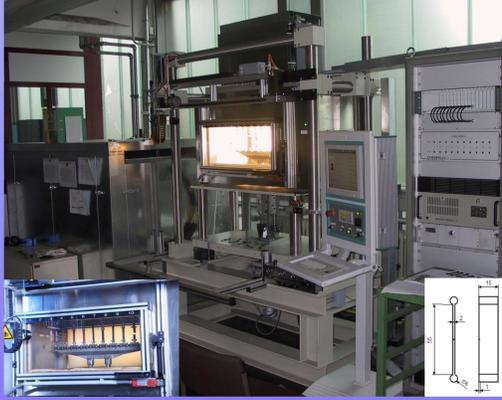
Photos of used Tear Analyzer System, temperature chamber with 10 test specimen installed some at different minimum loads and a sketch with test specimen dimensions.
