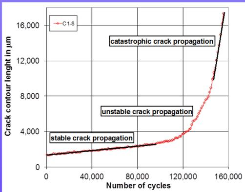
Typical crack contour length dependence on number of cycles for a carbon black filled EPDM, tested with pulses of 50ms, at 10Hz, 20% and 2N minimum load. Only the stable crack propagation region was used for this work.
