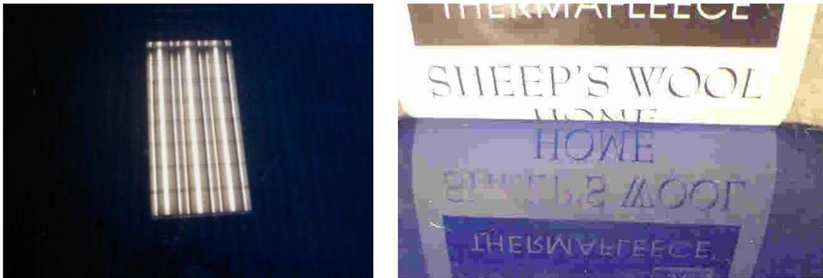
Figure 2: Reflection of a light fitting (left) and a packaging label (right) on the surface of a pigmented IMGC RIFT II plate.
