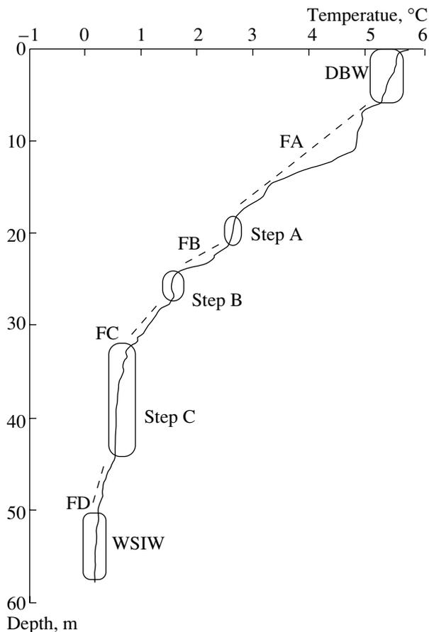
**Fig. 4.** Temperature profile at station 42, showing the mixing region marked as anomaly fluctuations FA, FB, FC, and FD, and identified water masses along with previously mixed water from observed quasi-homogeneous layers (Steps A, B, and C).
