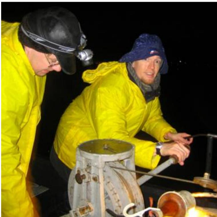
**Figure 7** F. Wobus (right) and local assistant Misha (left) lower the Niskin bottle to a set depth using the manual winch on the night cruise.
