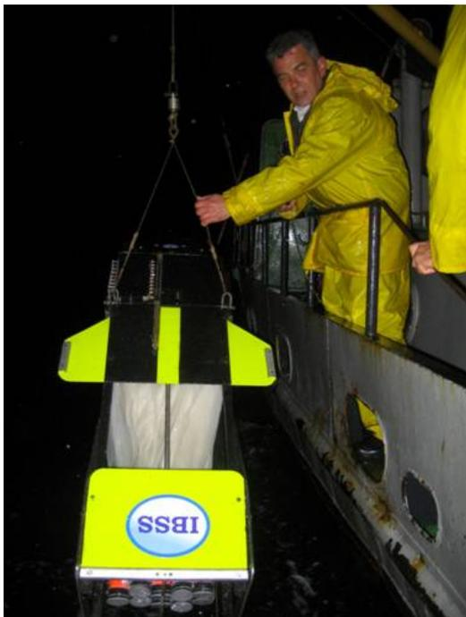
**Figure 5** The mechanical plankton sampler is deployed on the night cruise.
