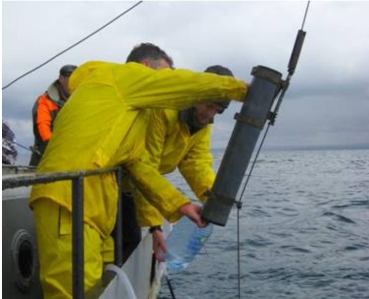
**Figure 6** V. Melnikov and F. Wobus retrieve a water sample from a Niskin bottle.
