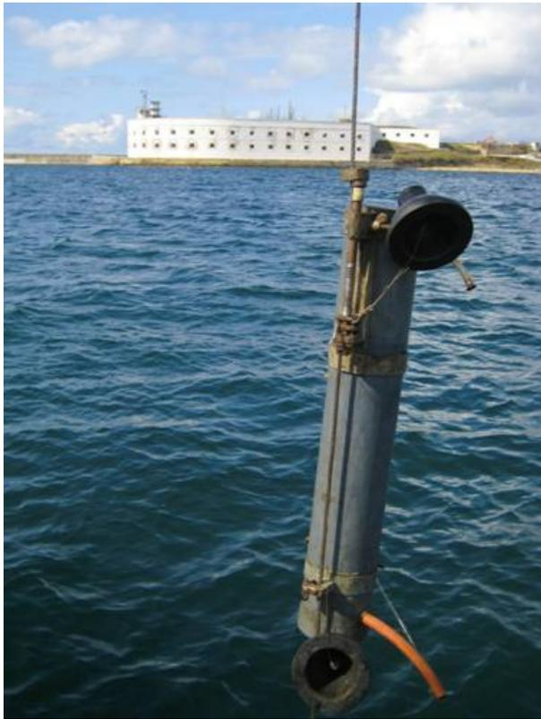
**Figure 2** Niskin bottle pictured in front of the historic Constantine battery in the bay of Sevastopol.
