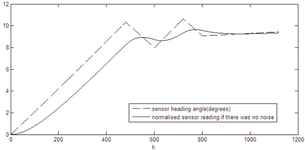
Figure 5, showing the response of the compass to an evolving heading angle, where the response has been scaled to match the input.
