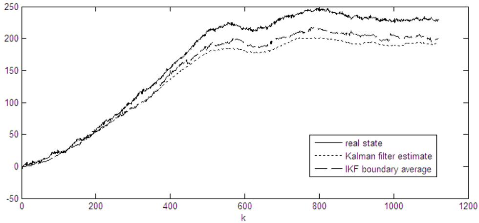
Figure 10, mid-values of the IFK intervals shown in figure 9, along with true state evolution and ordinary KF estimate.
