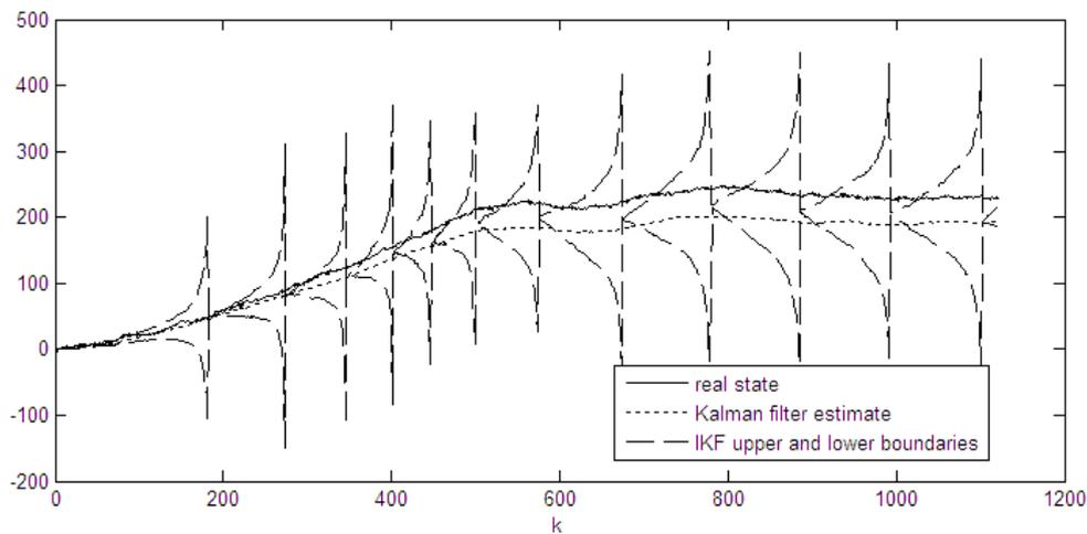
Figure 9, IFK boundaries using reset mechanism with a threshold value of 500, shown together with true state evolution and ordinary KF estimate.
