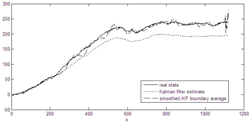
Figure 15, smoothed version of the mid-values of the IFK estimate of figure 14, shown together with true state evolution and ordinary KF estimate.
