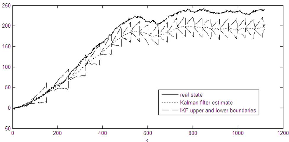
Figure 7, IFK boundaries using reset mechanism with a threshold value of 50, shown together with true state evolution and ordinary KF estimate.
