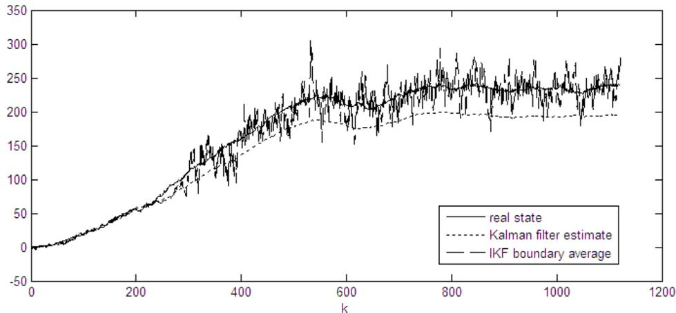
Figure 14, mid-values of the IFK intervals using percentage reduction mechanism with a threshold value of 50 and reduction parameter of 90%, shown together with true state evolution and ordinary KF estimate.
