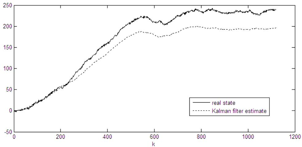
Figure 6, comparison of true state estimate and KF estimate: the KF estimate diverges from the true state because of the incorrect system model used in the filter equations.
