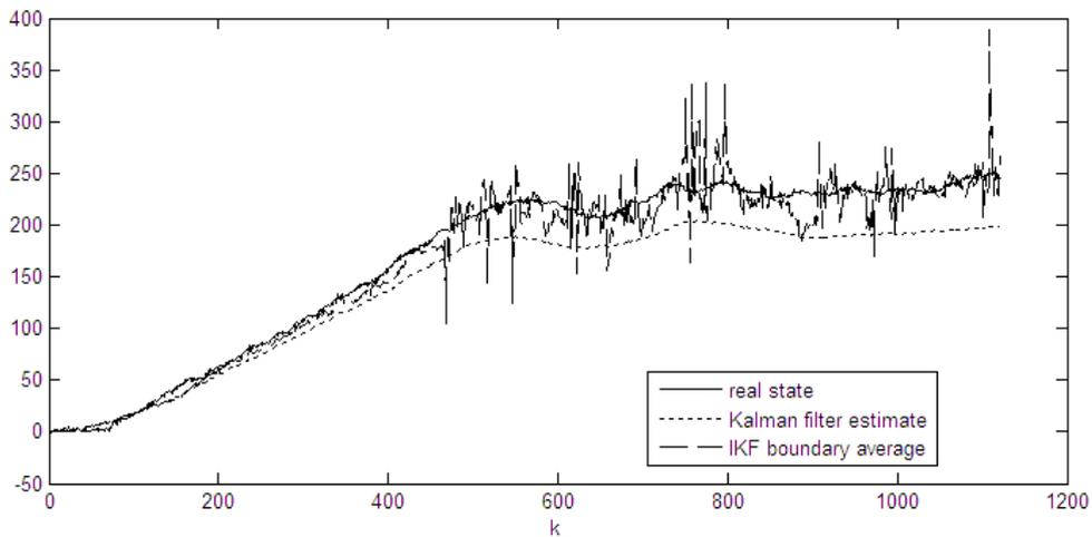
Figure 11, mid-values of the IFK intervals using reset mechanism with a threshold value of 5000, shown together with true state evolution and ordinary KF estimate.
