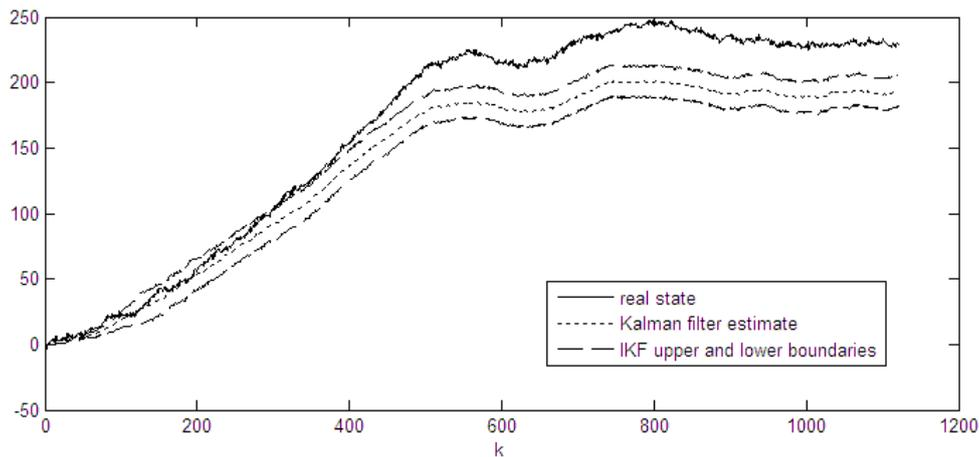
Figure 16, boundaries of the IFK intervals using percentage reduction mechanism with a threshold value of 25 and reduction parameter of 90%, shown together with true state evolution and ordinary KF estimate.
