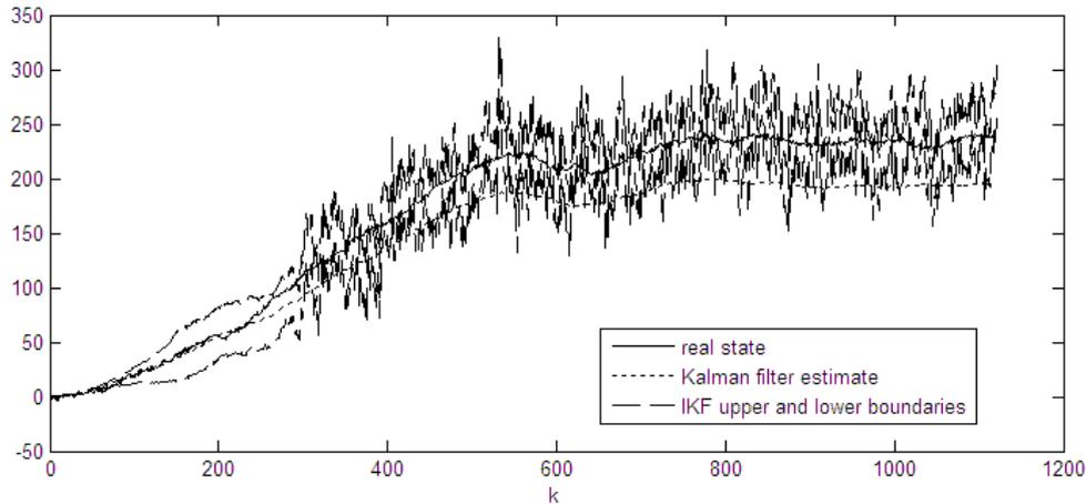
Figure 13, boundaries of the IFK intervals using percentage reduction mechanism with a threshold value of 50 and reduction parameter of 90%, shown together with true state evolution and ordinary KF estimate.
