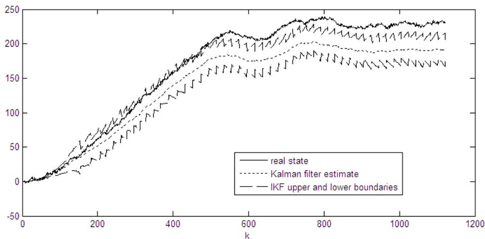
*Figure 12, boundaries of the IFK intervals using percentage reduction mechanism with a threshold value of 50 and reduction parameter of 50%, shown together with true state evolution and ordinary KF estimate.*
