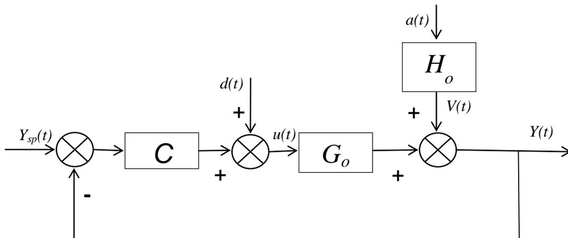
Figure 6: Closed loop system identification
