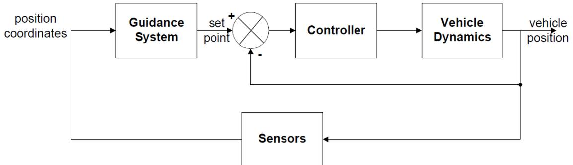
Figure 1: Guidance and control for a vehicle
