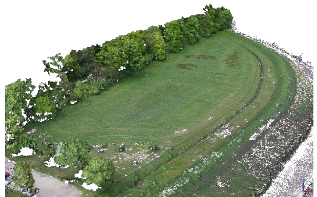
Above: UAV photogrammetry used to create a detailed 3D topographic surface
