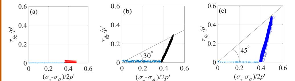
Fig.8 Stress paths in the normalised shear stress deviatoric stress plane for (a)  $\alpha_{sc} = 0^\circ$ ; (b)  $\alpha_{sc} = 15^\circ$ ; and (c)  $\alpha_{sc} = 22.5^\circ$ . (Laboratory test results)
