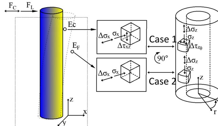
Fig.3 Schematic diagram of the pile-soil interaction with an HCTA sample positioned in front of the pile.
