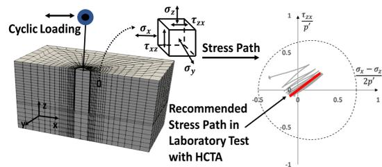
Fig.1 3-D Finite element model and stress path on soil elements.
