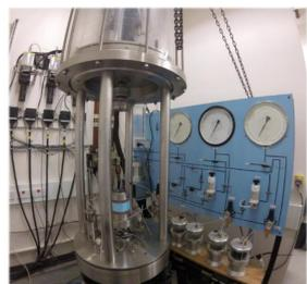
Fig.2 Hollow cylinder torsional apparatus
