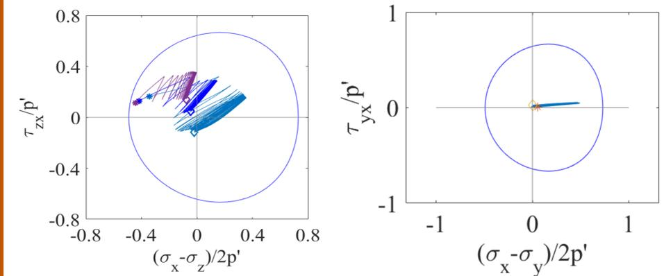
Fig.7 Normalised shear stress against deviatoric stress plot with results from soil element. (Numerical results)
