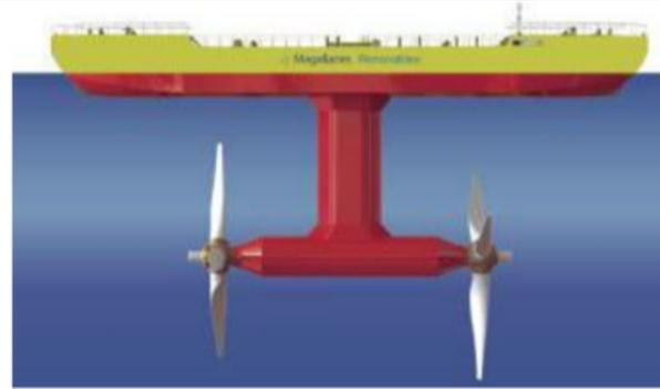
Figure 1. Schematic side view of the Magallanes ATIR rotor.
