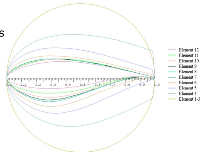
Figure 2. Blade profile along the radius of the Magallanes ATIR rotor.
