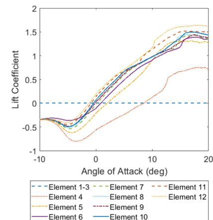
Figure 3. Lift coefficients for different elements along the radius of the rotor
