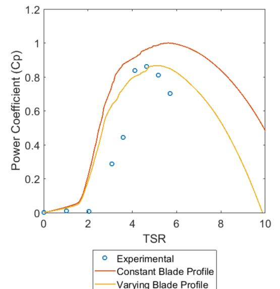
Figure 4. Comparison of coefficient of power against tip speed ratio for experimental and BEMT results.
