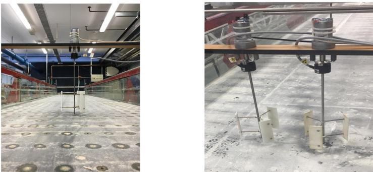
Figure 2. Experimental setup photographs of 1 turbine (left) and 2 turbines tested with lateral spacings of 1.5D and 2.0D (right).
