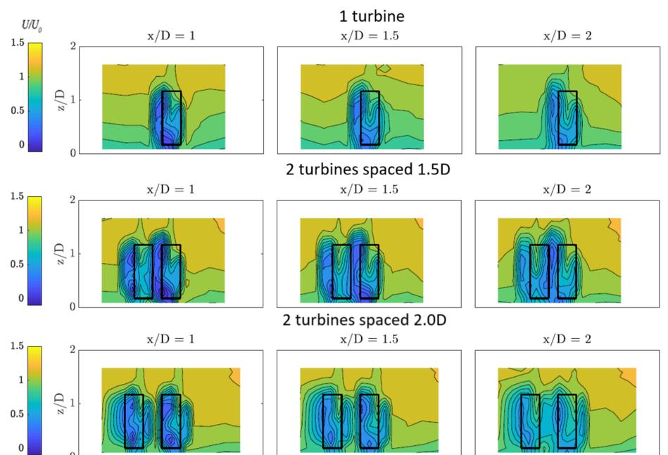
Figure 4. Contours of mean velocities ( $U/U_0$ ) at three cross-sections at  $x/D=1.0, 1.5$  and  $2.0$  for three cases with one turbine and two turbines laterally spaced by 1.5D and 2.0D. Rectangular box outlines indicate the location of the turbines
