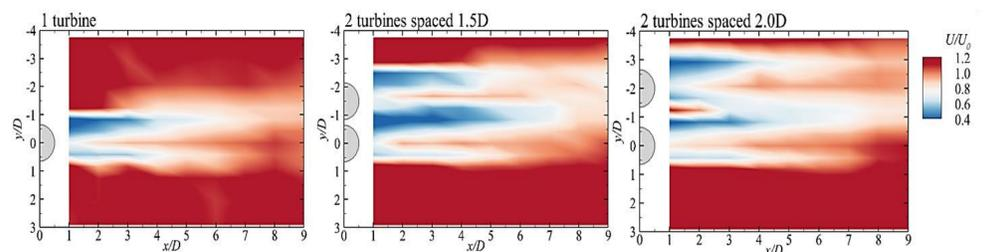
Figure 3. Mean longitudinal velocity fields ( $U/U_0$ ) across the channel width for three cases with one turbine and two turbines laterally spaced by 1.5D and 2.0D.
