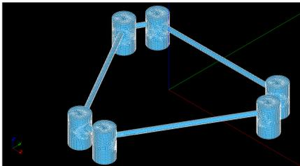
Figure 1: The fine mesh of the platform in Salome-Meca [4]
