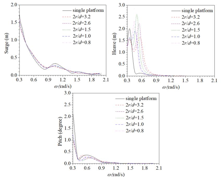
Fig. 4 Motion response of Windfloat platform versus  $\omega$  with different  $2r/d$
