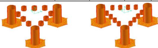
Fig. 3 Mesh of the hybrid system for two different layouts of WECs.
