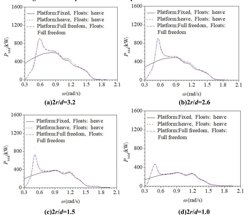
Fig. 5 Wave power with the fixed, heave motion and full freedom platform of different layout.
