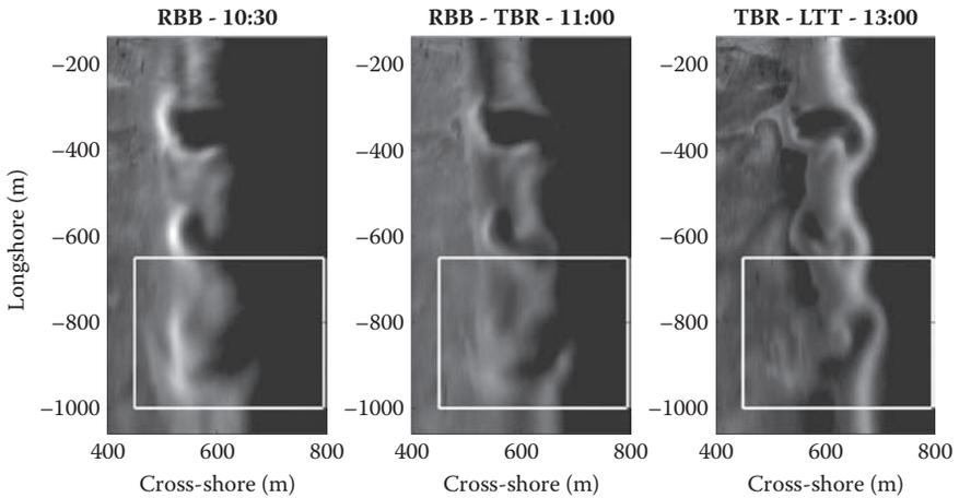
**FIGURE 14.10** Time-averaged plan view video images of Perranporth Beach, west Cornwall, taken August 3, 2008 at the times indicated above panels (cross-shore distance increases to seaward). High pixel intensities (whiter regions) indicate high wave dissipation (breaking). Panels show progressive change in effective morphological beach state from RBB to TBR/LTT during falling tide. The highlighted boxes indicate the regions of GPS drifter deployment shown in Figure 14.11.
