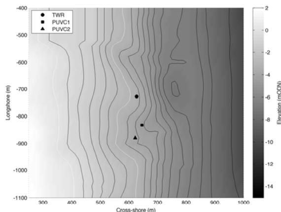
Figure 1. Combined results of the intertidal RTK-GPS survey and nearshore bathymetry indicating the instrument positions. Shading and contours indicate water depth (mODN; Ordnance Datum Newlyn). White contours indicate the mean low water spring (-3 m) and mean sea level (0 m).
