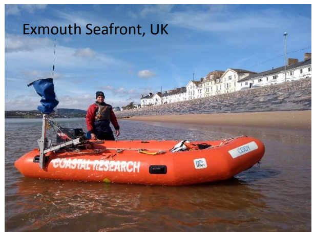
Above: RV Cody our inshore survey vessel with RTK GPS and single beam echo sounder
